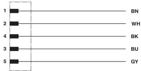
Contact assignment of the M12 connector
